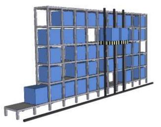
Fig. 2. A view of unit-load, crane-based, dual-shuttle, fixed aisle AS/R
