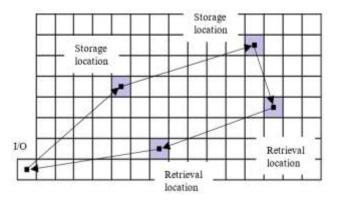
Path of the AS/RS machine consist of six locations defined as  $(X_m, Y_m)$  where  $(X_0, Y_0)$  is starting point, from  $(X_1, Y_1)$  to  $(X_4, Y_4)$  are storage/retrieval points and  $(X_5, Y_5)$  is finishing point. The travel distance which begins from I/O station, including the storage/retrieval points and finishes I/O station is calculated by (1). Starting location and finishing location are the same location.
