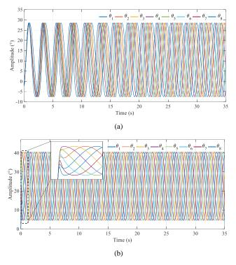
Fig. 8. Joint angles of the turning motion: (a) Hopf, (b) ACP
