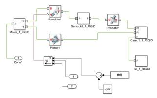
Fig. 4. MATLAB/SimMechanics model of a link of the snake robot
