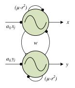
Fig. 2. Hopf oscillator structure
