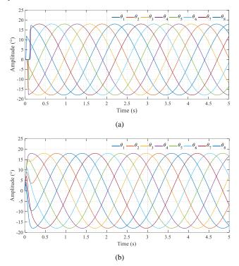
Fig. 6. Joint angles of the forward motion: (a) Hopf, (b) ACP
