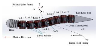
Fig. 3. The designed snake robot model
