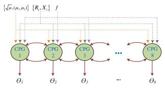
Fig. 5. CPG network structure with bidirectional coupled scheme
