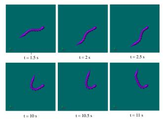
Fig. 10. Snapshots of SimMechanics for forward and turning motions of the snake robot. It is noticed that After 10 s, bias is set to 1.25
