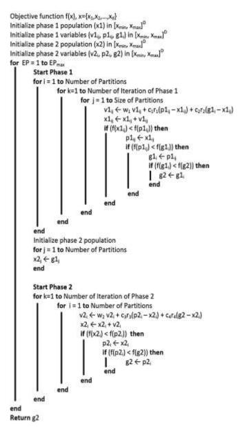
Fig. 1. Implementation of GSO algorithm with PSO
