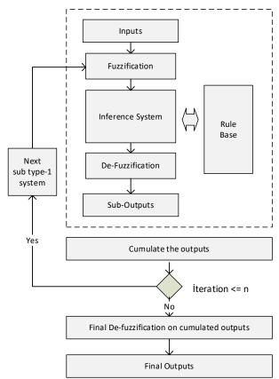
Fig. 7. Block diagram of nonstationary fuzzy system mechanism.
