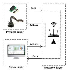
Fig. 1. The block diagram which shows simply how a CPS works [2].
