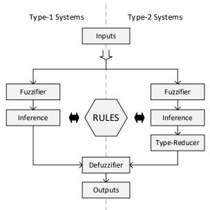
Fig. 5. A block diagram for type-1 and type-2 fuzzy system steps.
