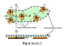
In this study, we has developed a software that shows data and the insole placed in shoes for the use in gait analysis of Internet of Things.The sensors in the developed zone are connected wirelessly via Bluetooth, communicating with mobile devices or PC, and displaying incoming graphs.
