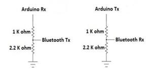
Fig 9. HC-05 Module Connection with Arduino
