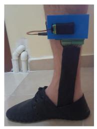
Fig 12. Wearable Kinetic IoT System
