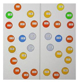
Fig 16. Average force generated by sensors during walking
