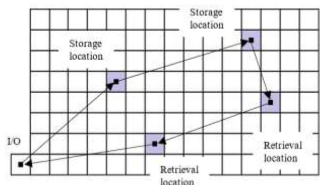
Path of the AS/RS machine consist of six locations defined as  $(X_m, Y_m)$  where  $(X_0, Y_0)$  is starting point, from  $(X_1, Y_1)$  to  $(X_4, Y_4)$  are storage/retrieval points and  $(X_5, Y_5)$  is finishing point. The travel distance which begins from I/O station, including the storage/retrieval points and finishes I/O station is calculated by (1). Starting location and finishing location are the same location.
