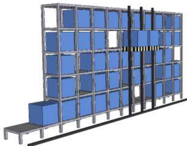
Fig. 2. A view of unit-load, crane-based, dual-shuttle, fixed aisle AS/RS
