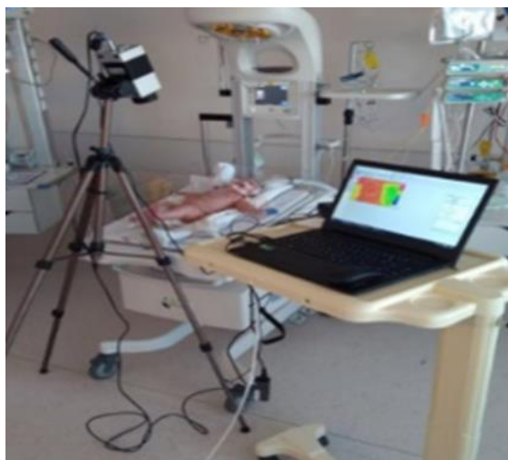
Fig. 1. Thermogram acquisition procedure [6].
