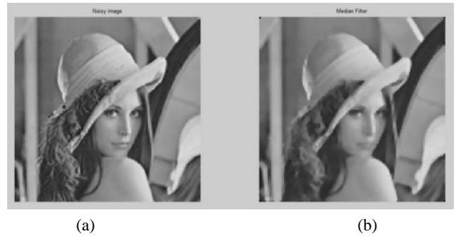
Fig. 7 : (a) Noisy Image (b) Filter Image using Median Filter
