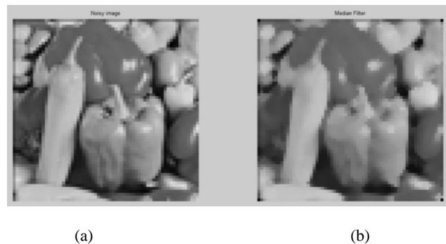
Fig. 8: (a) Noisy Image (b) Filter Image using Median Filter
