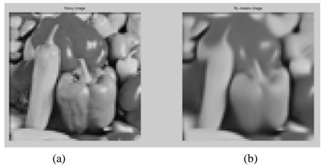
**Fig. 14:** (a) Noisy Image (b) Filter Image using NLM Filter
