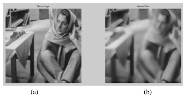
Fig. 9: (a) Noisy Image (b) Filter Image using Wiener Filter
