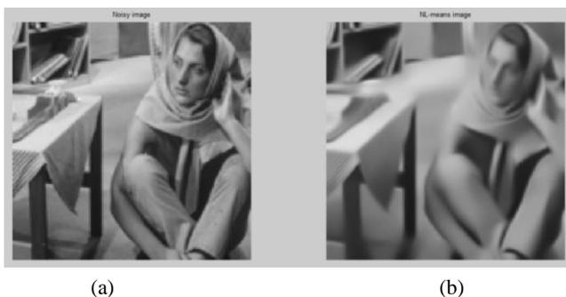
**Fig. 12:** (a) Noisy Image (b) Filter Image using NLM Filter
