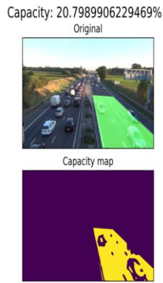
Figure 6- Generated Capacity map sample result2
