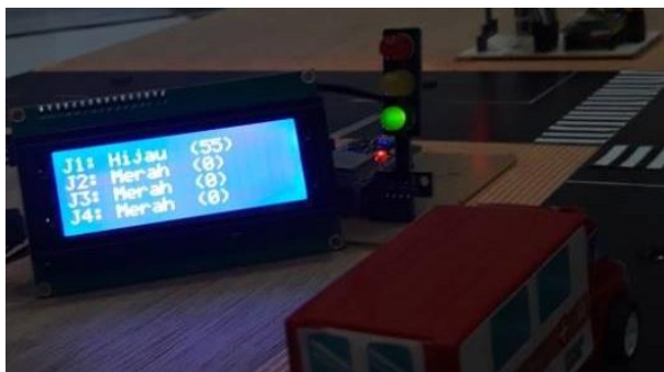
Figure 15 LCD Display during Traffic light control
