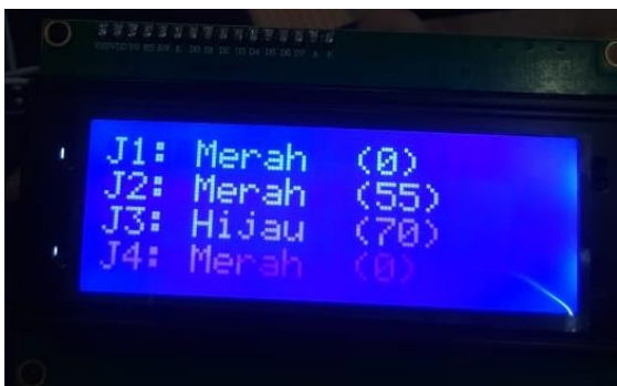
Figure 18 LCD Display during collision involving the same vehicle types
