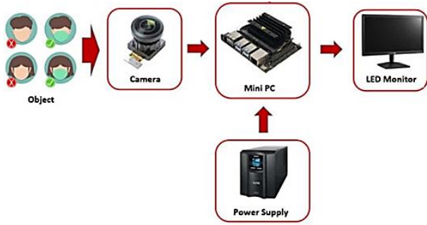
Figure 2. Block diagram of mask detection system.
