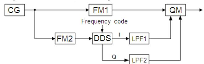
Figure 1 – Block diagram of the quadrature signal generator of the UAV payload radio transmitter
