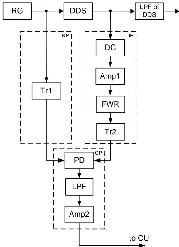
Figure 2 - Block diagram of the ACPD control signal formation path
