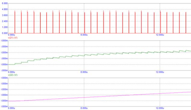
Figure 8 - Waveforms of signals at the output of the control path links (from top to bottom): phase detector FD, low-pass filter LPF2 and amplifier A3
