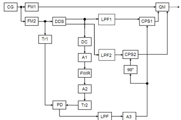
Figure 3 – Block diagram of the payload signal generator of the UAV radio transmitter with an autocompensator of phase distortion
