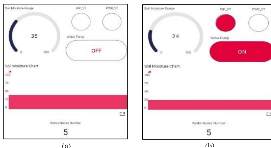
Figure 8 (a) work of the irrigation system in the Blynk server
