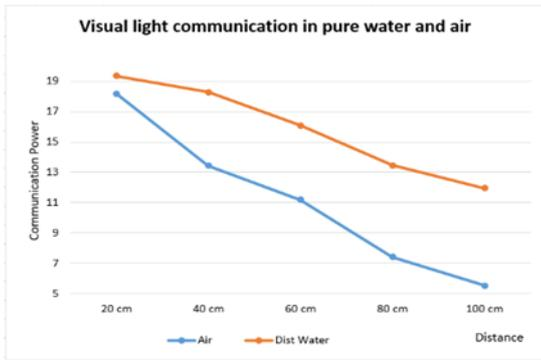
**Fig. 5.** Visual light communication performance in pure water VS air.
