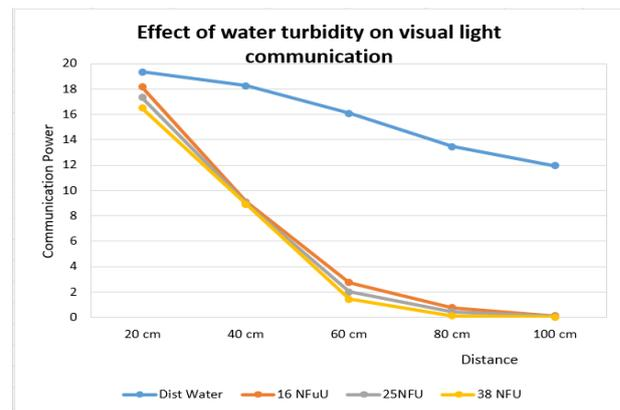
**Fig. 9.** Effect of changing turbidity on UWVL communication.
