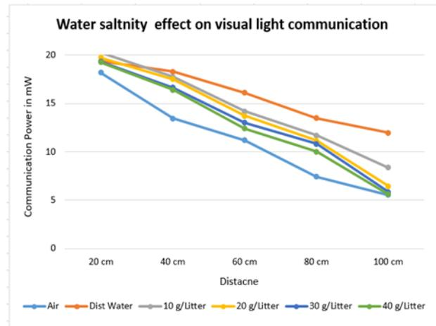
**Fig. 7.** Overall effect of increasing water salinity on UWVL communication under different mediums.
