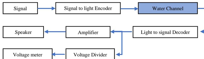
**Fig. 4.** Underwater visual light communication system block diagram
