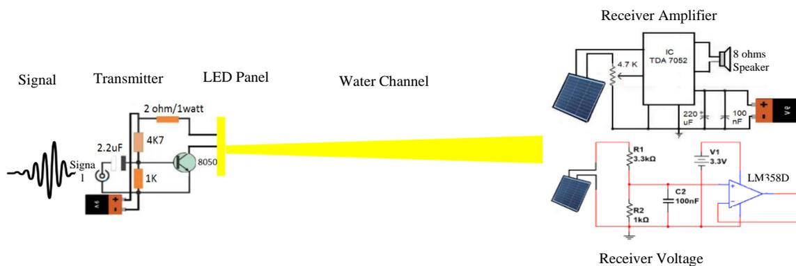
**Fig. 3.** Underwater visual light experimental setup
