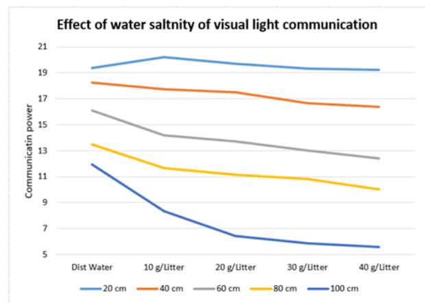
**Fig. 8.** Overall effect of increasing water salinity on UWVL communication under varying distances.
