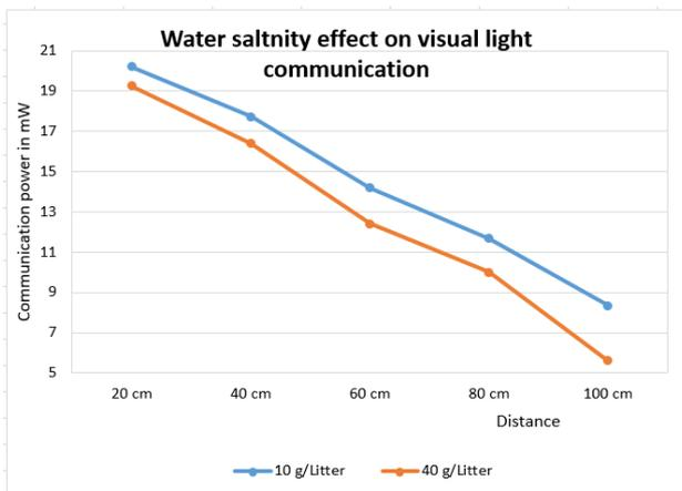
**Fig. 6.** Effect of water salinity on underwater visual light communication.
