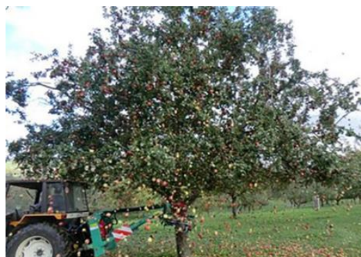
Fig. 4. Trunk shaker harvesting example[17] (Courtesy Feucht Obsttechnik GmbH Company)
