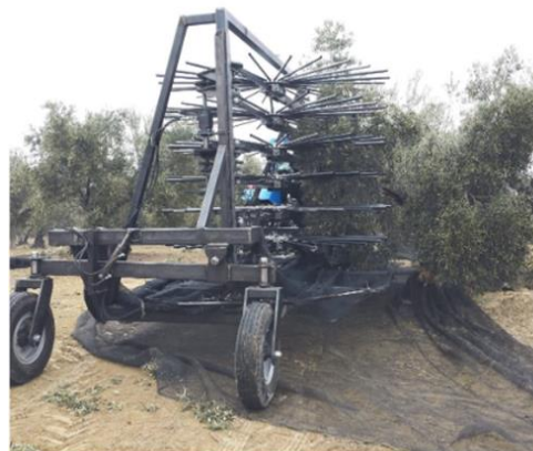
Fig. 3. Canopy shaker example.[16]
