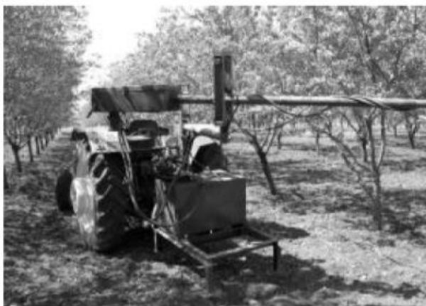
Fig. 2. Limb shaker example.[15]
