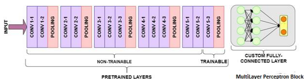
Fig. 8. Layered architecture of proposed DCNN model
