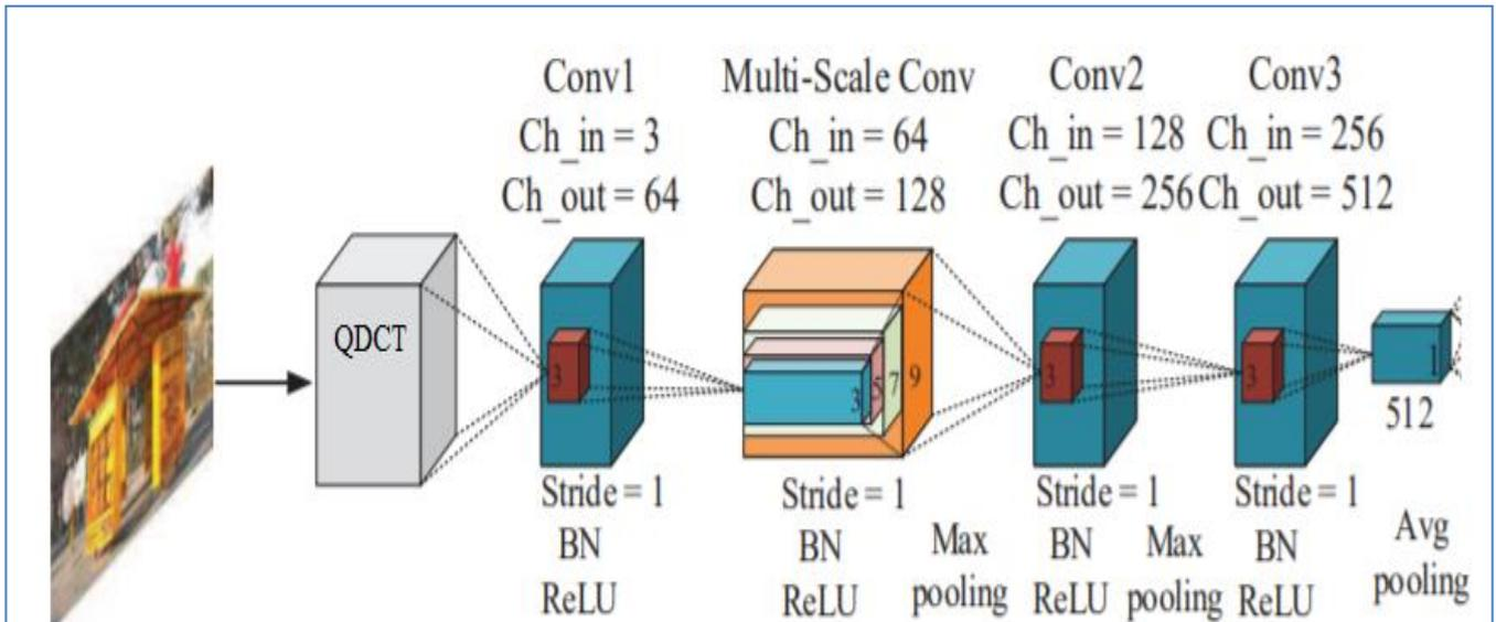
**Fig. 2** QDCT CNN for feature extraction
