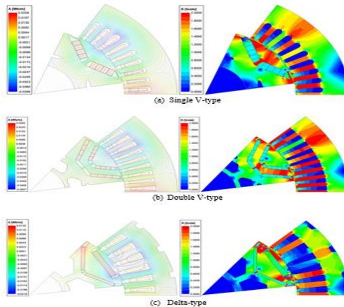
**Fig 2.** Magnetic flux density and Magnetic flux diagram for each model.
