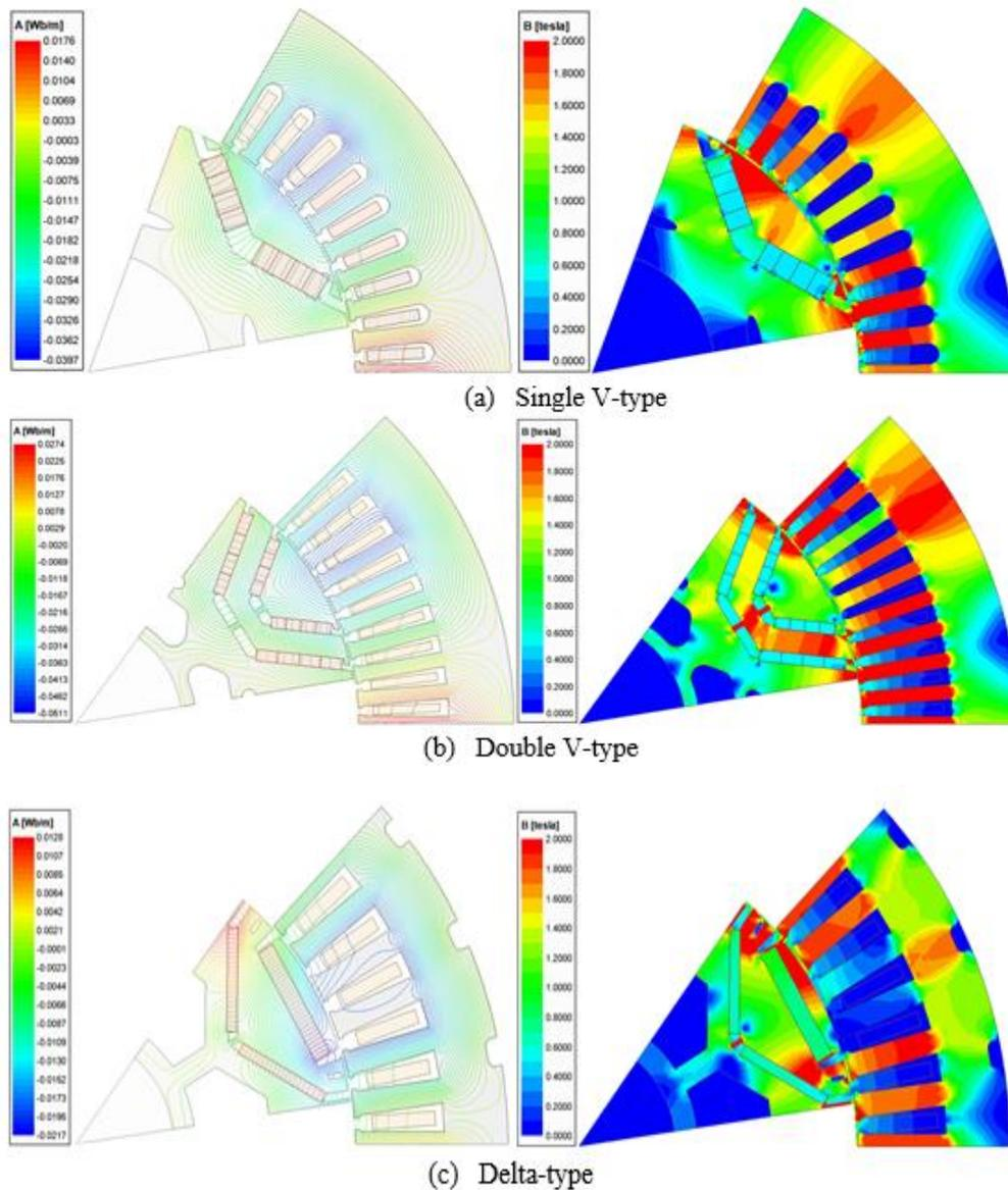
**Fig 4.** The magnetic flux density and magnetic flux diagram of each model with the Rib removed.
