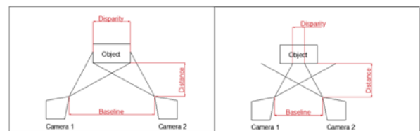
Fig. 1. Relation between disparity and baseline
