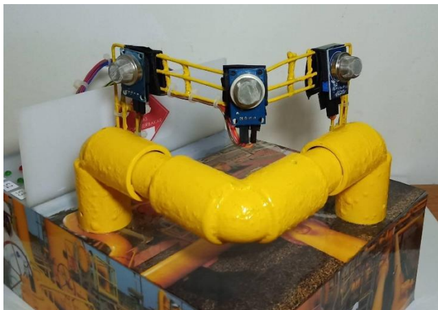
Fig 15. The installation of MQ-4 gas sensor and other components
