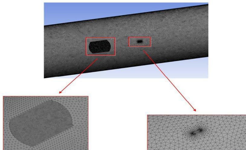
Fig. 2: The pipeline grid division. Refinement of the corrosion defect grid in part and Refinement of the grid at the crack
