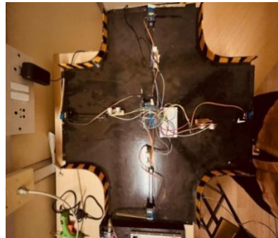
Fig 1 fixing sensors at the junction of the bridge
