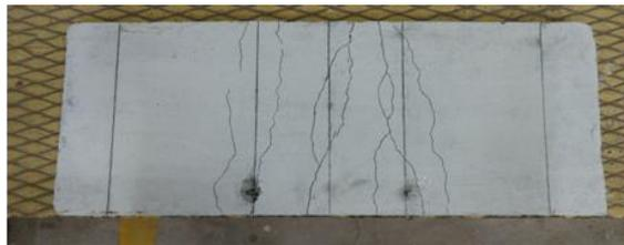
**Fig 3.** Crack patterns in slab panels
