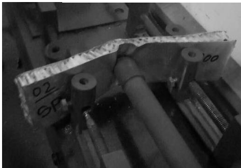
Figure 7 Specimens' deformation in bending configuration
