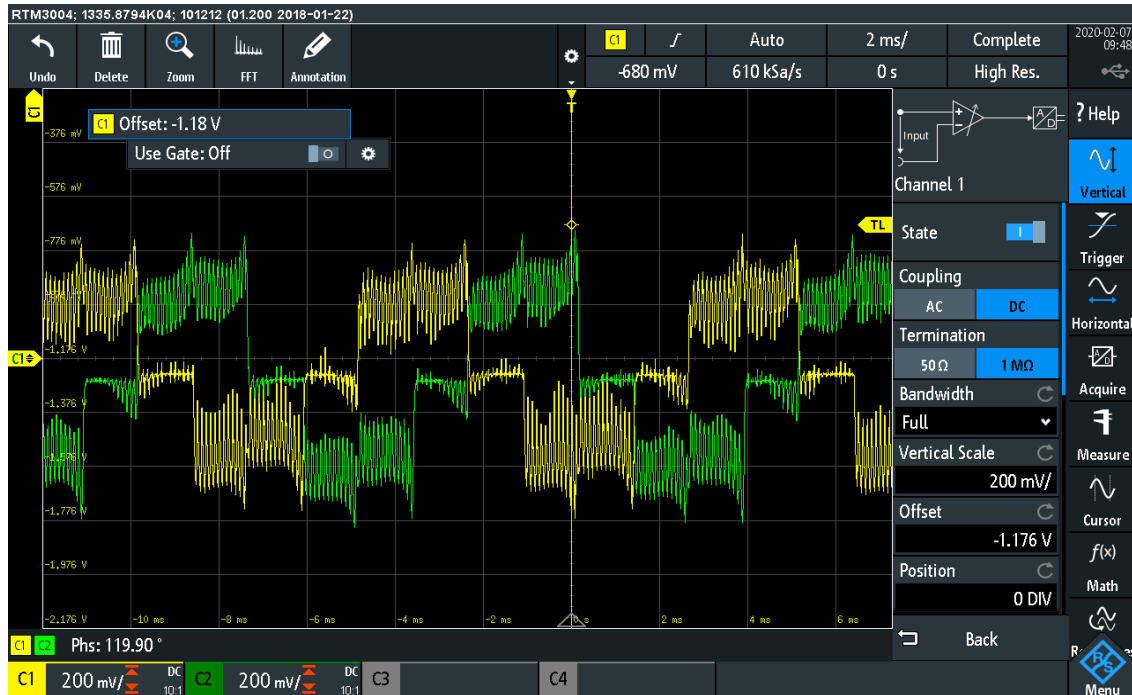
Fig 5. BLDC Experimental Parameters (a) Input Current ( I_r & I_y ) .
