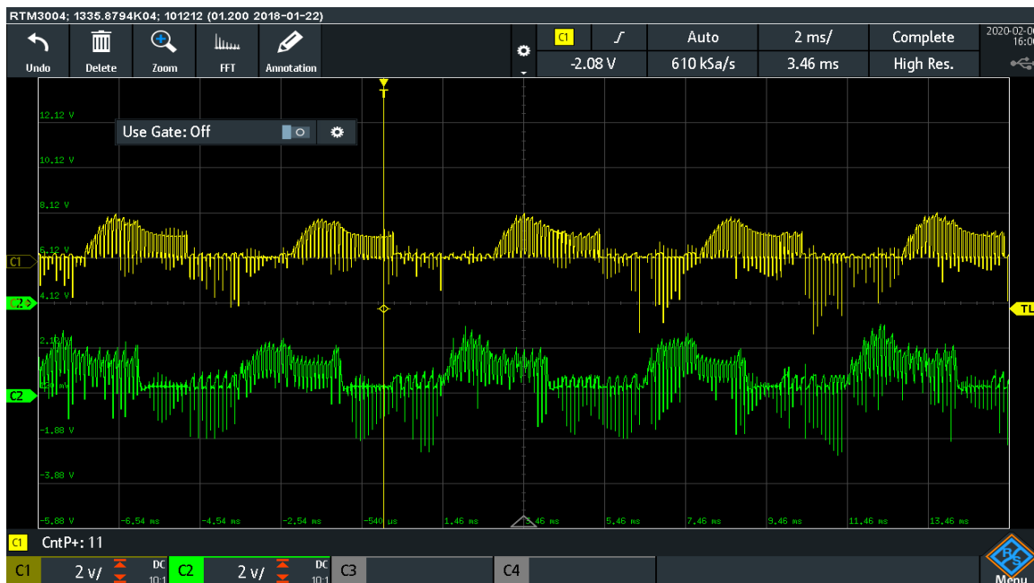
Fig 7. SRM Experimental Parameters (a) Input Current (Ia & Ib).
