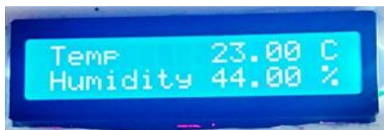
Figure 2: Display the values of Temperature & Humidity
