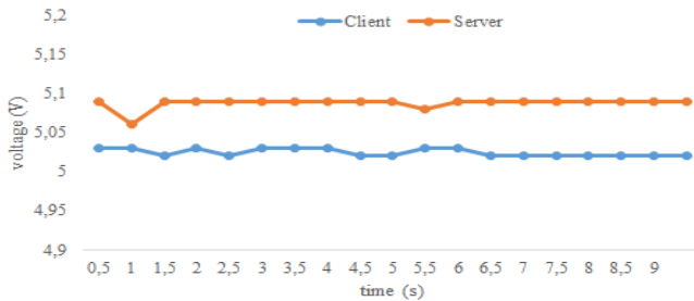
Fig 8. Comparison of voltage consumption between the client and server
