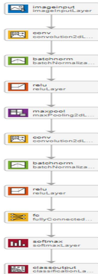
Fig. 3. Convolutional neural network architecture.
