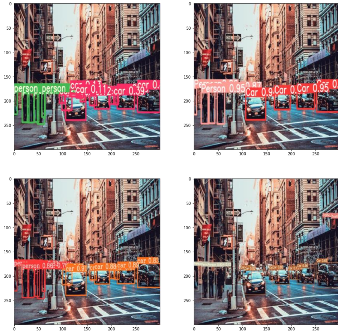
Fig5. From top left to bottom right, i) YOLOR ii) YOLOv5 iii) YOLOv6 iv) YOLOv7 Alt Text: 4 different algorithms detecting objects of different classes in a different lighting scenario, helping us to validate the results and select the best algorithm.
