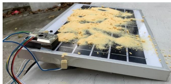
Fig. 6. The dirty solar panel testing.
