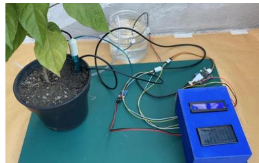
Fig. 4. Prototype of smart farming system with the irrigation unit
