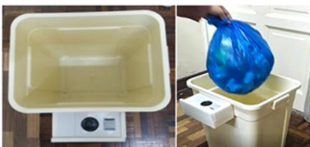
Fig. 15. The garbage bin started to fill with trash and the distance detected is displayed on the Blynk app.
