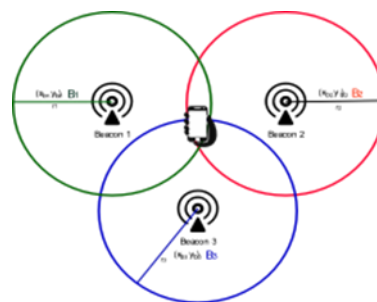
Fig 7. The concept of trilateration
