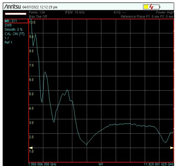
Fig.16 VNA results of VSWR Plot of Fabricated Antenna
