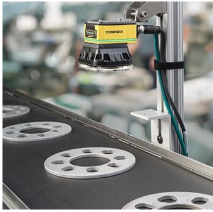
Fig. 1. Mechanical product surface fault detection machine running on conveyor
