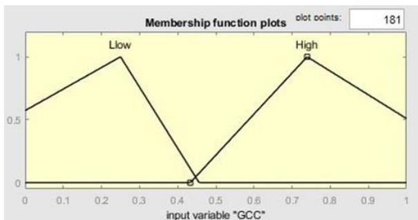
**Fig. 4.** Input set of the fuzzy inference system - GCC.
