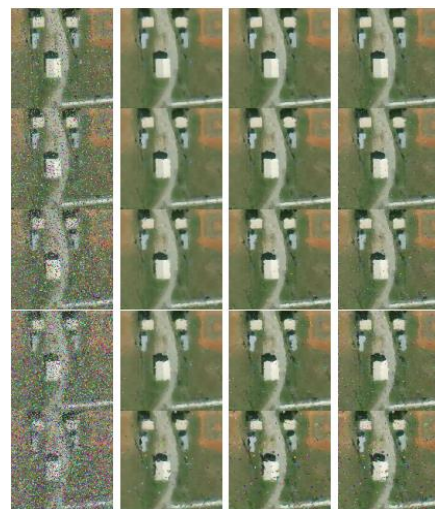
Fig. 2. The filtered results of the SAT-1 image. A noisy, ARWSF, DOAF, and FDOAF image is shown from left to right. Starting at the top: p = 0.1, 0.2, \dots, 0.5 .
