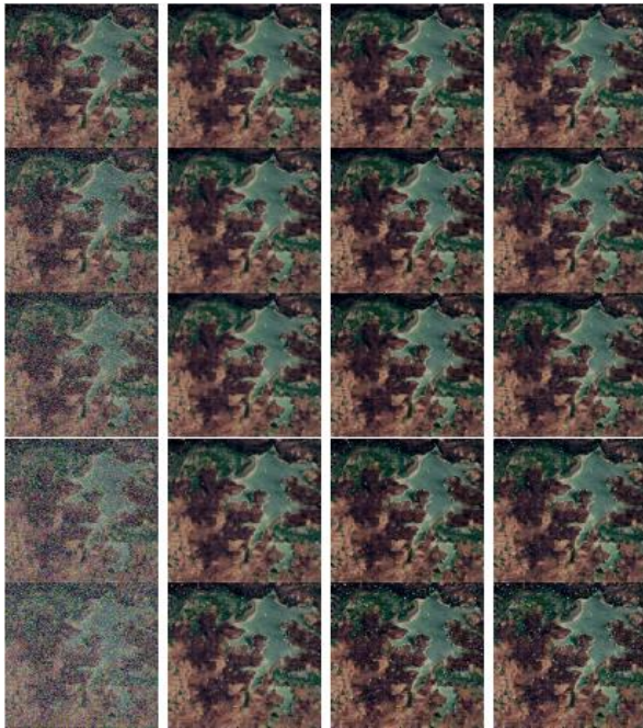
Fig. 3. The results of the SAT-2 image filtering. From left to right, noisy, ARWSF, DOAF, and FDOAF p = 0.1, 0.2, \dots, 0.5 from top to bottom.
