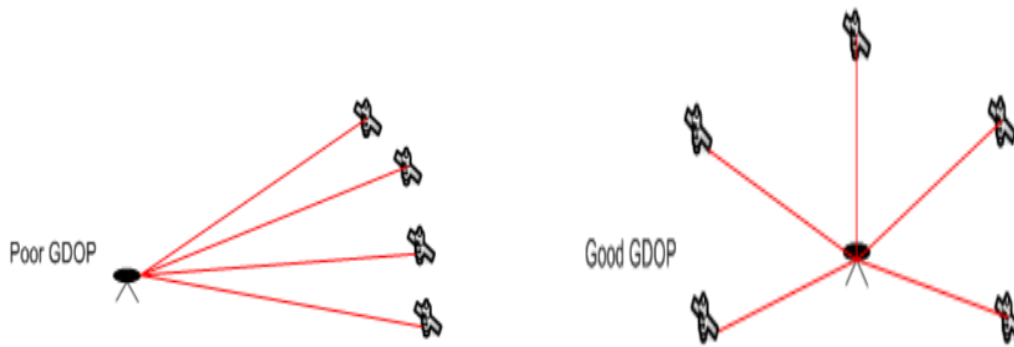
Fig 4: The above diagram indicated how the distribution of satellites will result in good GDOP.
