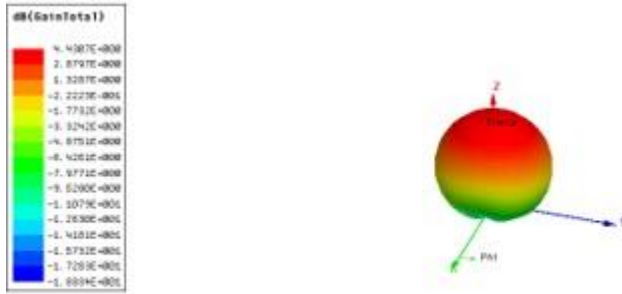
Fig 8: Gain for slotted antenna for modified Dumbbell shaped slotted antenna with rectangular DGS.
