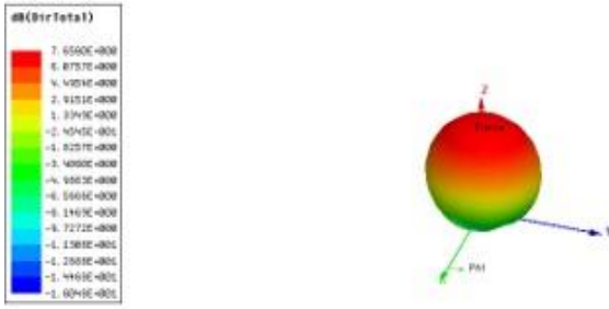
Fig 19: Directivity of modified Dumbbell shaped slotted antenna with Elliptical DGS.
