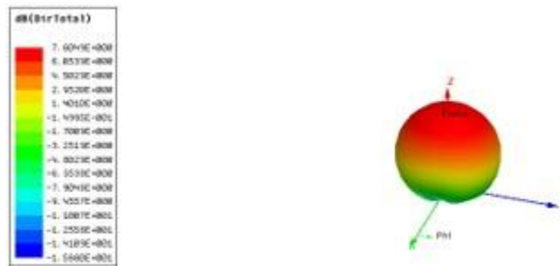
Fig 9: Directivity for slotted antenna for modified Dumbbell shaped slotted antenna with rectangular DGS.
