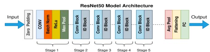
Fig 1. ResNet50 model Architecture [33]
