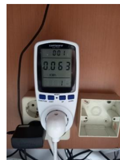
Fig 9 Power Monitoring Device
