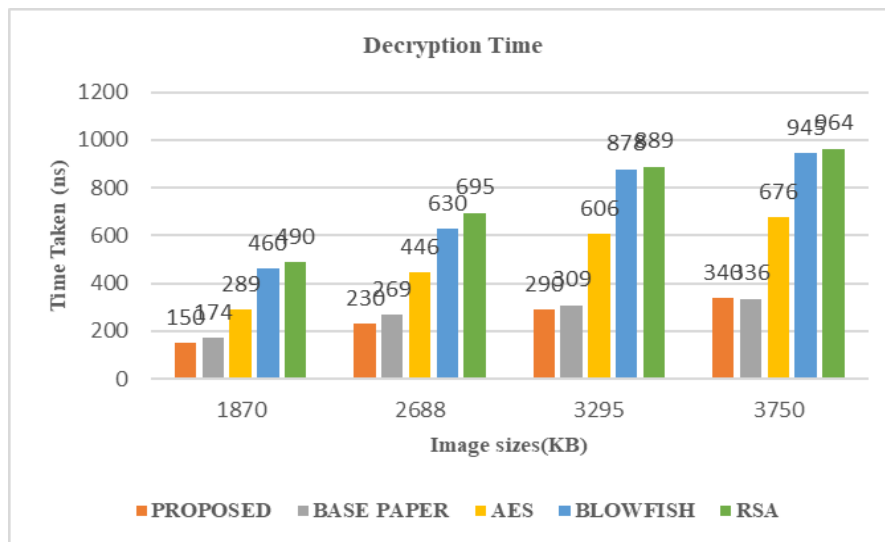
Fig. 7. Comparison of Decryption Time Between Proposed and Existing Algorithms Across Various Image Sizes
