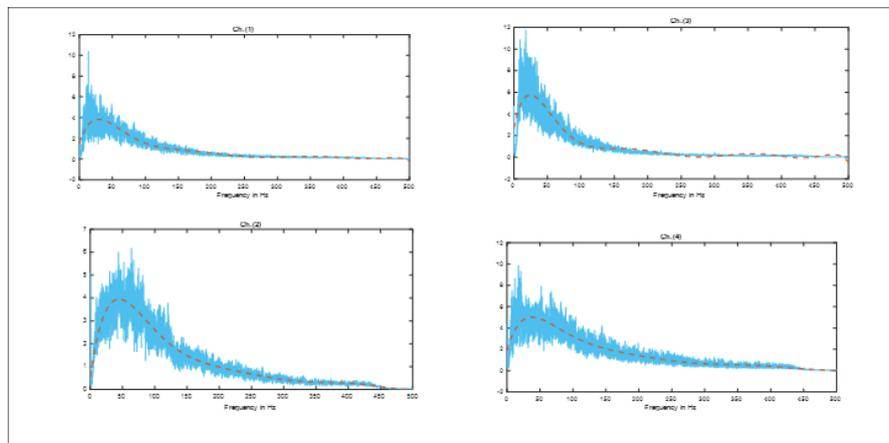
**Fig (3.a).** Average of Normal EMG spectrum and it's mean
