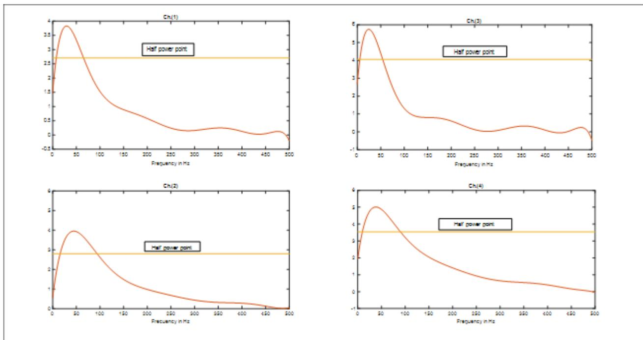
**Fig. (4.a)** Mean of EMG spectrum and its half power points for Normal cases (CH.1,2,3,4)
