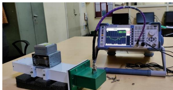
Fig. 2. Testing of magnetron launcher and coaxial adapter using VNA (R&S-ZVL model).
