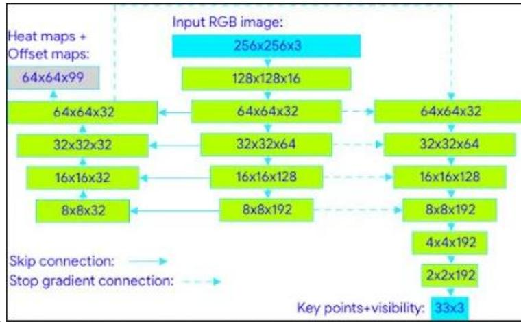
**Fig. 3** Blazepose model architecture
