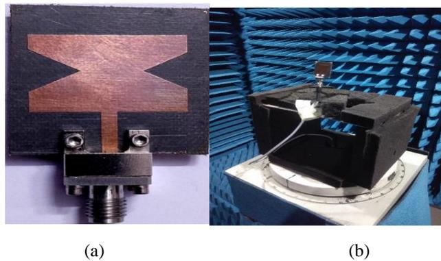
Fig 5. (a) Photographs of the fabricated prototype and (b) Antenna placement in an anechoic chamber.
