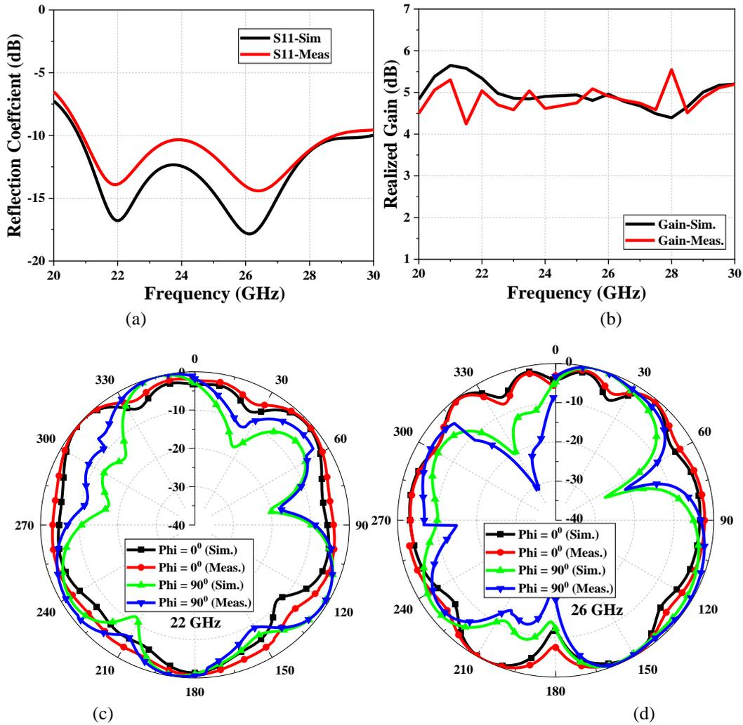
**Fig 6.** Simulated and measured: (a) Reflection coefficients vs frequency, (b) gain vs frequency, (c) radiation patterns at 22 GHz, and (d) at 26 GHz.
