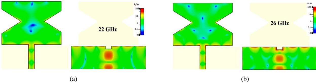
Fig 4. Surface current distribution at the chosen frequencies of 22 GHz and 26 GHz.
