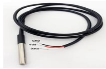
Fig 4. Water Temperature Sensor
