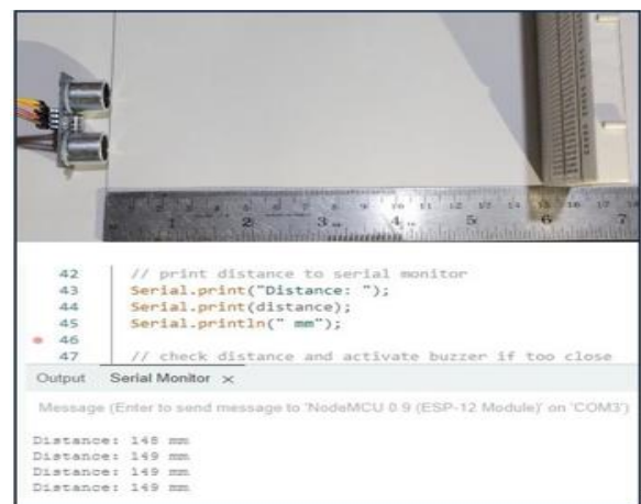
Fig.3. Accuracy testing for 150 mm distance.
