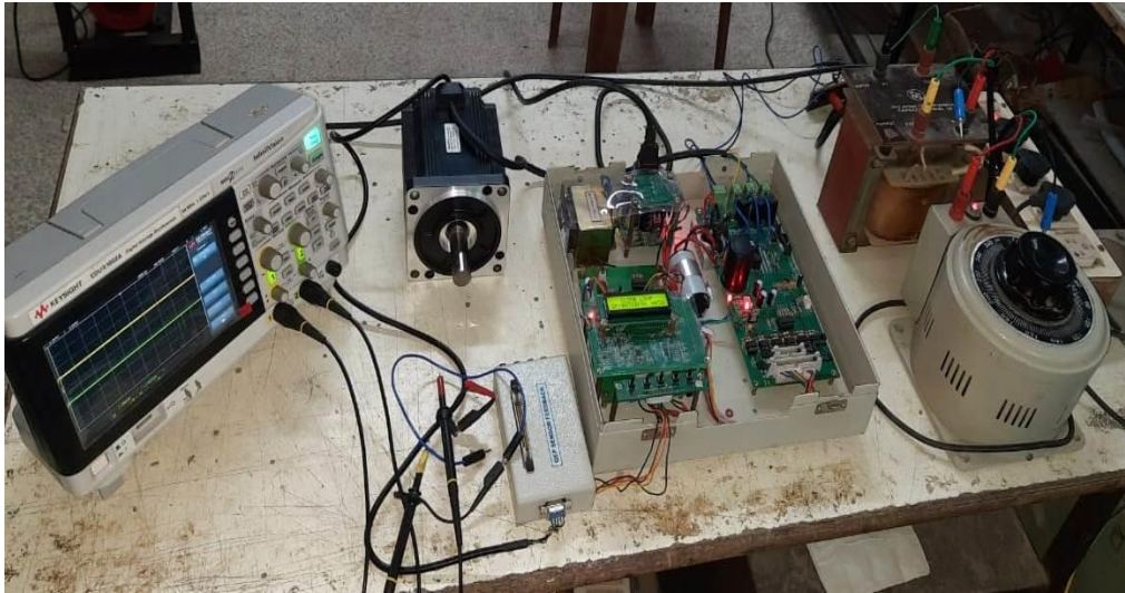
Fig 7. Proposed system power circuit with RP2040 controller.
