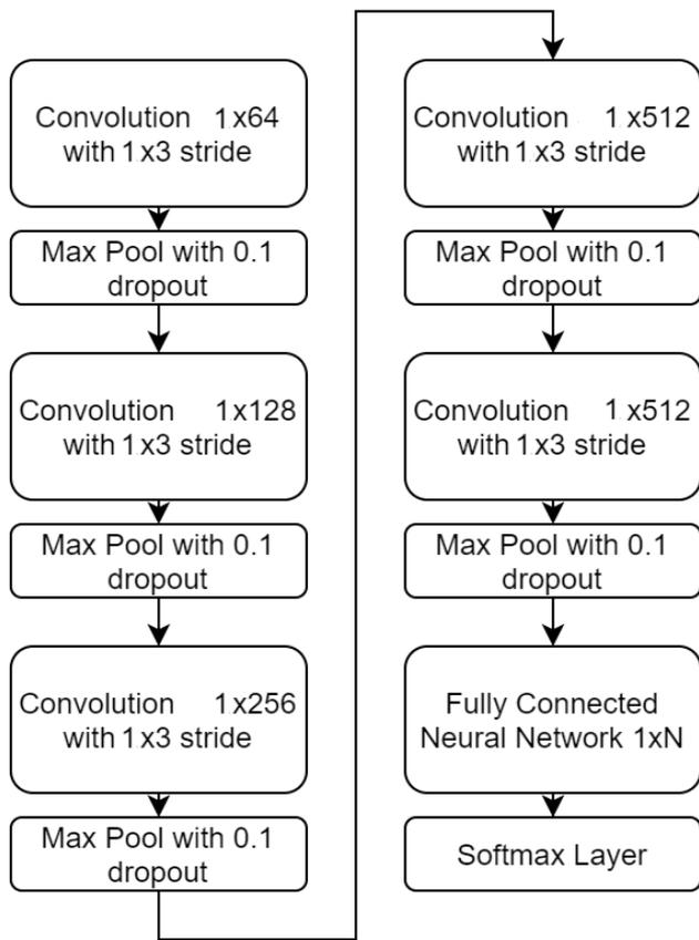
**Fig 1.2.** Design of the 1D CNN process
